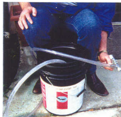
LOAD THE HOSE HOLDING THE QUIK GUN AT BUCKET LEVEL
